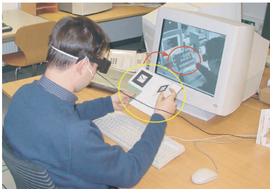
Fig. 4. A user working with our desktop VR system. A FireWire camera (out of view) is used for optical tracking of the hand held props which are equipped with markers (see yellow ellipse). The image of the camera is used as a video background. Stereoscopic images are displayed on the monitor which give the user who wears shutter glasses the impression of working in 3D space. The virtual images of pen and PIP can be seen on the monitor (red ellipse) as an overlay over the video image.
