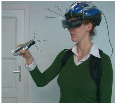
Figure 2: Outside view of a user constructing a solution. The user wears a head mounted display and uses a wireless pen as an input device.
