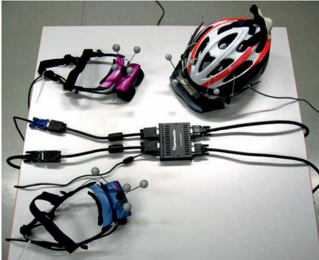
Fig. 2. One input and 3 output connectors. Three HMDs (two Emagin Z800 and one Sony Glasstron) are attached to the Matrox TripleHead2Go. In our 6-user setup three more Sony Glasstron HMDs were attached to another TripleHead2Go box.
